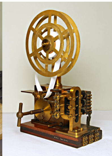
Ehrenhaft's three-lever recorder (original) and condenser (replica) from around 1914, kept by the Vienna Technical Museum.
