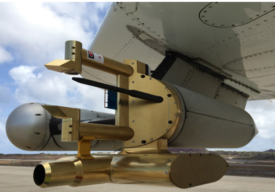
Fig. 1: The CAPS instrument of the AEP group mounted under the wing of the NASA research aircraft DC-8 during the ATom-2 mission in February 2017.
