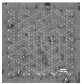
in the form of single flux quanta, the motion of these flux quanta can be used as a method to investigate the influence of the artificially created defect columns. The flux quanta are preferentially anchored in defects and since their motion causes dissipation, stable arrangements that impede motion lead to high critical currents and low resistance.
